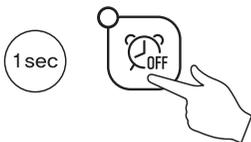
4. To cancel 'Off Timer', press and hold 'Off Timer' button for 1 second. It will then switch the timer off automatically.
